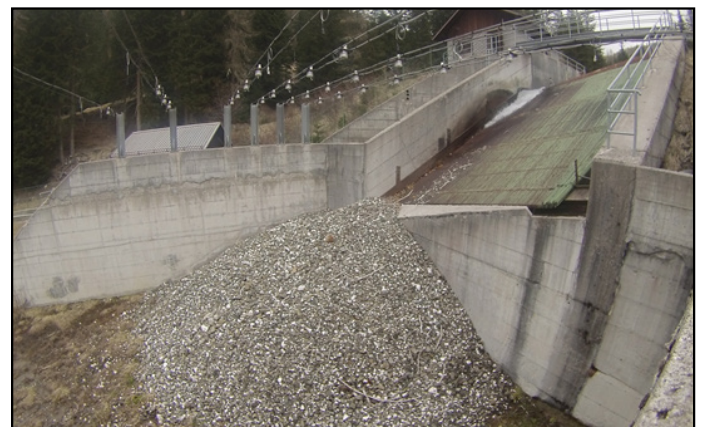
Figure 2. Bedload material is separated from the flow and collected in a pile. The pile is then surveyed for volume and grain size distribution. This data can be used to validate the geophone data.
