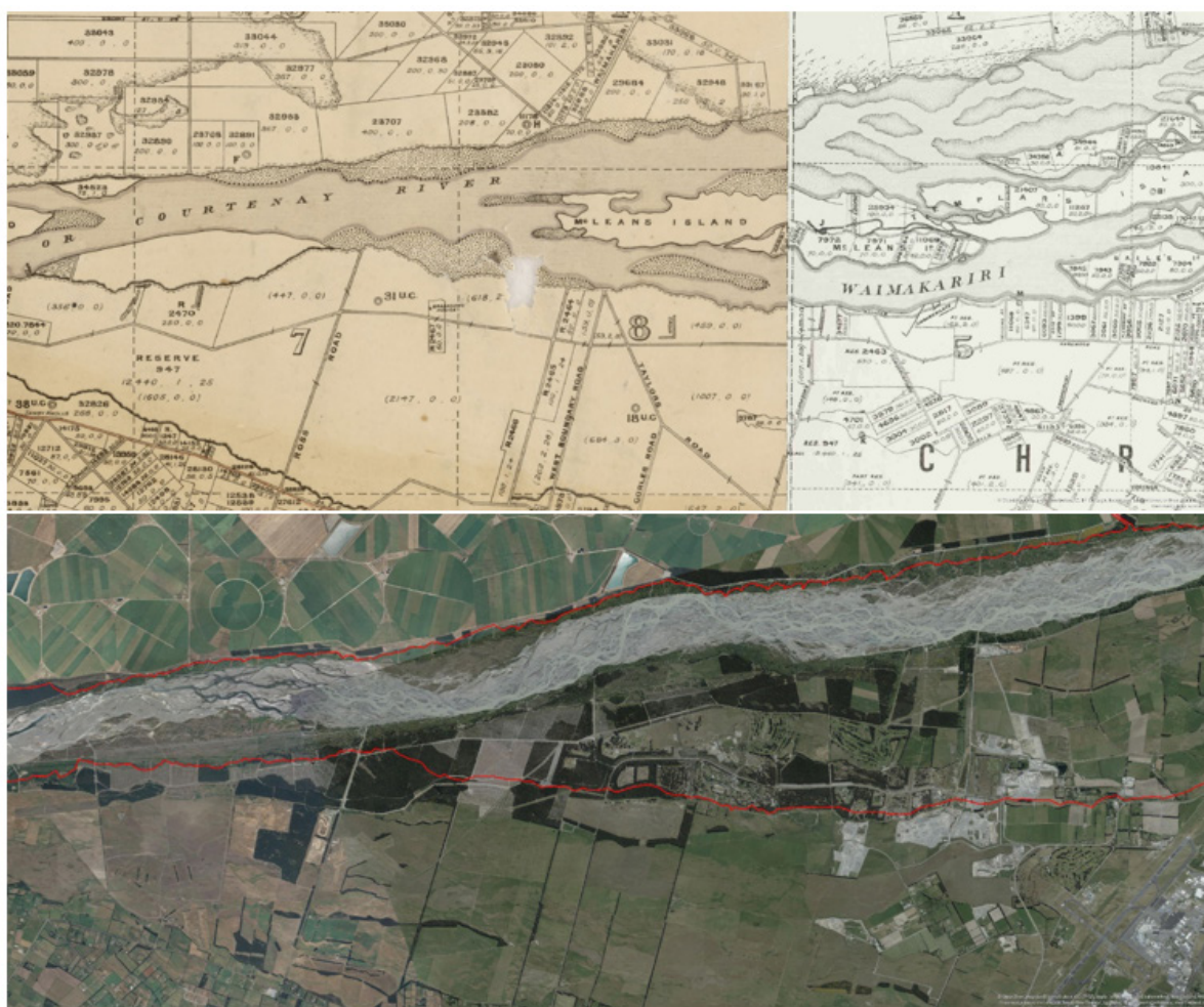
Braidplain delineation for a reach of the Waimakariri River. Top image shows the 1899 map and bottom shows the 2019 aerial with historical braidplain in red.
