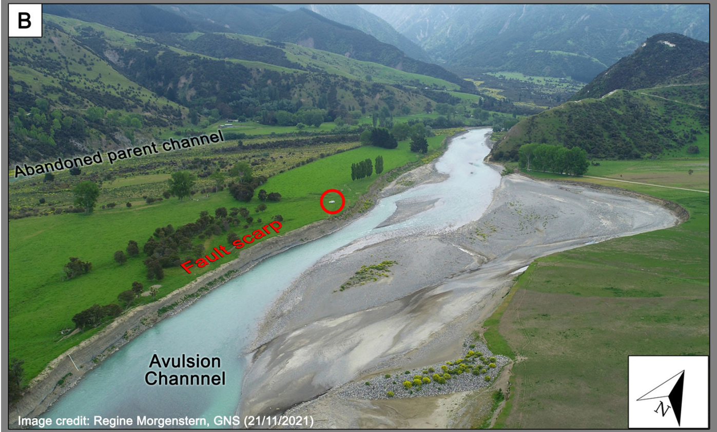
Figure 1A: The Papatea Fault rupture and Waiau Toa | Clarence River coseismic avulsion. The Papatea fault produced \sim 6.5 m of vertical, and \sim 4.6 m of lateral offset downstream of the river flow direction (shown by the arrows), causing the river to partially avulse (Image adapted from McEwan et al 2023).
