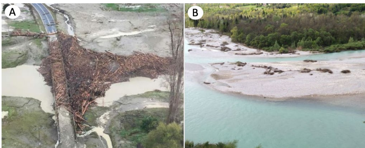
Figure 3. Instream wood accumulation at a bridge after a flood event occur in Gisborne, New Zealand (A); Instream wood deposited along channel bars and potential source of wood from the riparian area in Piave River, Italy (B).
