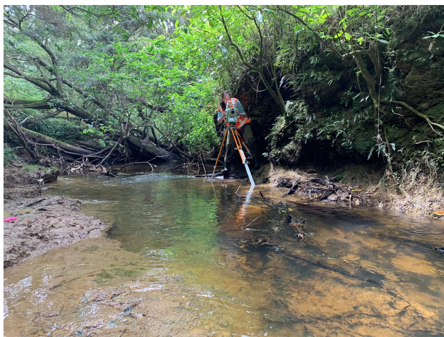
Jacqui McCord undertaking terrain laser scanning to assess fine grained geomorphic units within the Kourawhero Stream.
