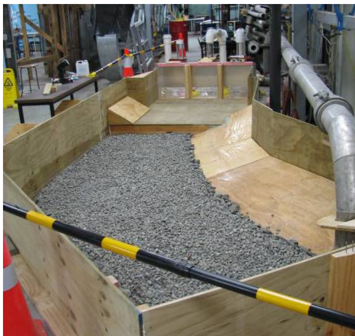
A Physical Model Aiding the Design of a Pump Station Intake (Geometric Scale 1:7.6)
