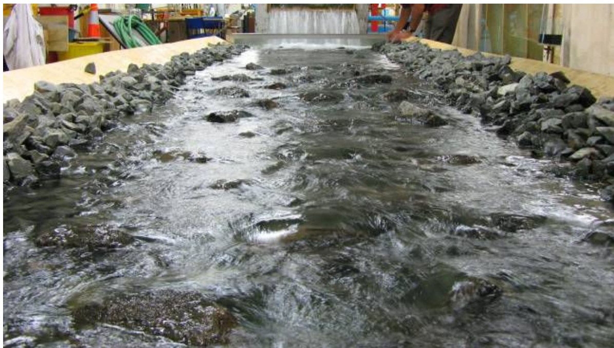
1:2 Scale Model of a Natural-channel Fish Pass Design
